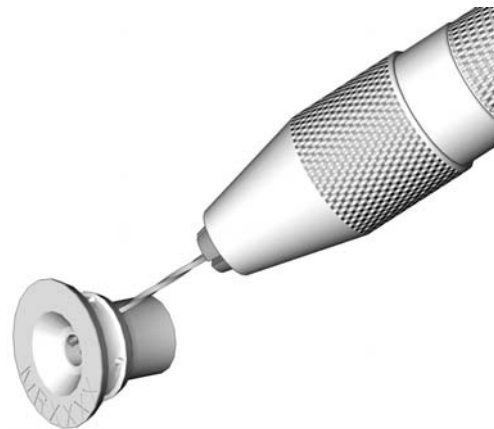
FIG. 2. Cleaning Component B (Resin) Ports
