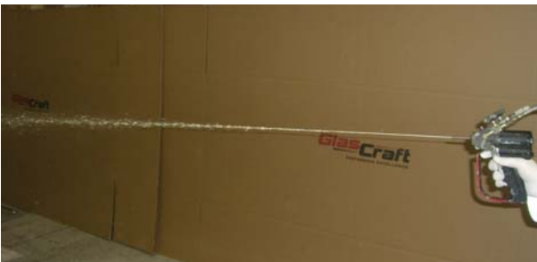
Stream Jet Application Up to 30' (10m)stream
